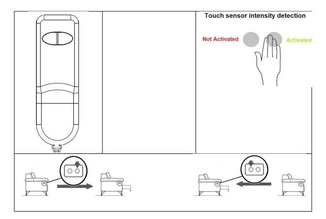
Extending the relax/sleep function - Hold down the button until the sliding mechanism extends and reaches the desired position and then release the button. The sliding mechanism will remain in the selected position.
